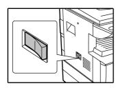
It will take about 45 seconds for the machine to warm up. While the machine is warming up, the POWER SAVE indicator (②) will blink. (The POWER SAVE indicator (②) will go off when the machine is ready to copy.)
